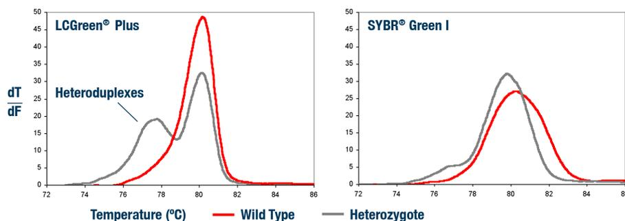
Derivative melting curves illustrate superior detection of heteroduplexes in the heterozygous mutant using LCGreen Plus, compared with negligible heteroduplex detection using SYBR Green I.
