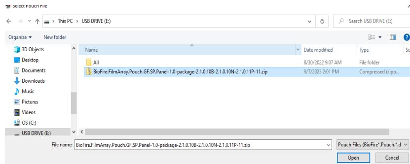
8. Verify the pouch module builds are correct. The BioFire GF SP Panel has three analysis packages with build versions that must match the screenshot below. If older builds were previously installed, they will automatically be replaced.
